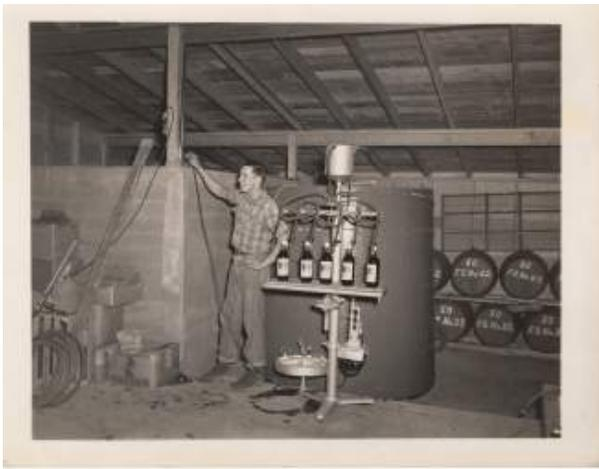
Photo courtesy of Rachael Woody A worker pours wine into bottles in this undated photo, using an early form of a bottling machine.
